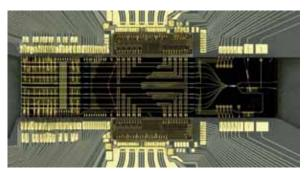
**Fig. 3:** 10 x 10 Gb/s tunable DWDM PIC, integrated with high-speed drivers (courtesy of Fraunhofer IZM Institute)
