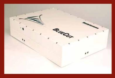
Figure 1: Shown is a picture the BlueCut laser head. Dimensions of the laser head are 325 x 445 x 110 mm<sup>3</sup>.
