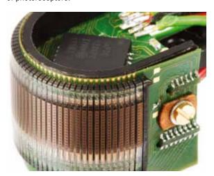
**Fig. 3:** Cylindrical curved multi-aperture navigation sensor (radius of curvature 6.35 mm).
