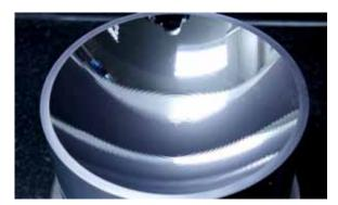
**Fig. 2:** Ultrasonic assisted diamond turned mold insert with superimposed microstructures for automotive industry
