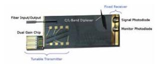
**Fig. 4:** Tunable 1-2.5 Gb/s bidirectional transceiver on Polymer motherboard (courtesy of Fraunhofer Heinrich-Hertz-Institute).
