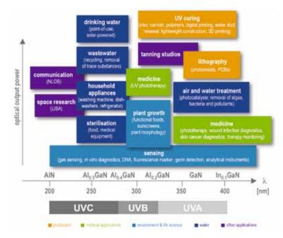
Fig. 1: Applications of AlGaN-based LEDs emitting in the UV-A (400nm-320nm), UV-B (320nm-280nm), and UV-C (280nm-200nm) spectral range. Source: FBH
