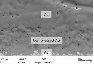
Fig. 1: Cross sections showing a nanoporous Au structure after etching selectively the Ag (left) and after TC bonding onto a substrate with Au metallization by applying a pressure of 50MPa at 250 °C (right).
