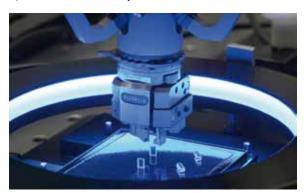
Fig. 2: Ultra precision multi-axis handling of micro-optical components
