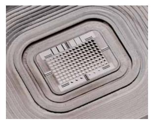
**Fig. 1:** Master of a single refractive freeform array fabricated by an ultra-precise machining process.
