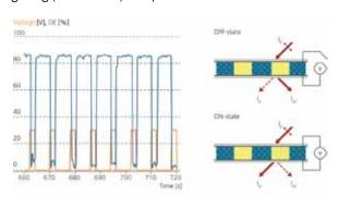
**Fig. 1:** ON/OFF electrical switching upon application of an electrical field and dependence of diffraction efficiency on applied electric pulses.
