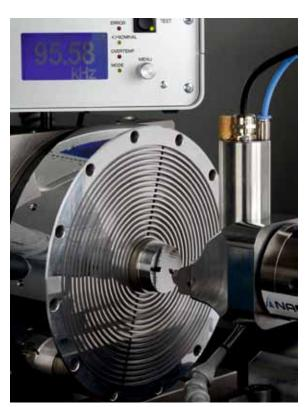
**Fig. 1:** Transversal ultrasonic oscillator ILSonic with a depth of penetration up to 70 mm at an operating frequency of 95 kHz
