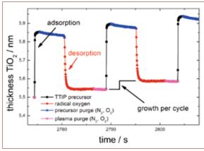
$\rm ALD$  process of  $\rm TiO_2$  deposition: Real time monitoring of adsorption, desorption and purging processes during ALD cycles
