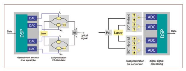
Fig. 2: Schematic setup of an optical software-defined multi-format transponder (left: Tx part, right Rx part).
