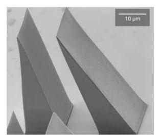
Fig.3: Photonic structures with a large aspect ratio and extraordinary steep flanks
