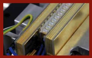
High-power diode laser stack delivering 3 kW output power, suitable for pumping of solid-state lasers. Source: ©FBH/P. Immerz
