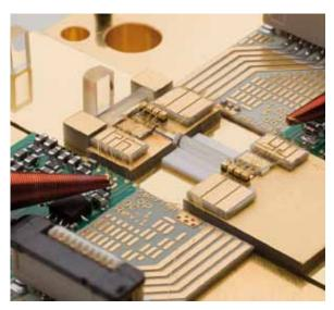
Pulsed laser system including GaN transistors (FBH technology). Source:  $\ensuremath{\mathbb{C}}$  FBH/schurian.com
