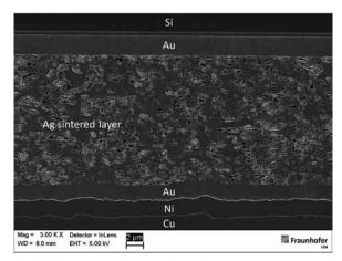
**Fig. 3:** Cross sections showing a Si die Ag sintered on a Cu substrate (with a noble metallization each) by applying pressure of 10 MPa pressure at 230 °C.
