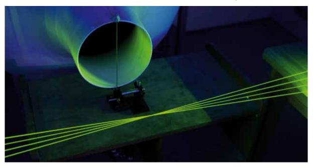
classical optical instruments like microscopes. They also enable highly innovative systems using adaptive optics as demonstrated in the experimental setup for 3d airflow measurement from Prof. Czarske.
