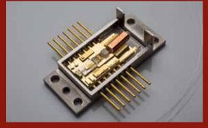
Miniaturized laser module for efficient fiber coupling of highpower diode lasers. Source: ©FBH/schurian.com
