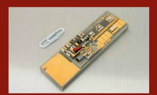
Hybrid-integrated MOPA module for atomic spectroscopy in space. Source: ©FBH/P. Immerz
