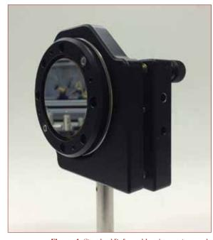
**Figure 1:** Standard Deformable mirror setup ready for integration.
