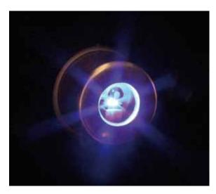
Blue-emitting GaN laser diode with 440 nm in TO housing. Source: © Philipp Keshet
