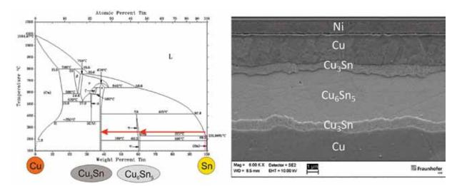
Fig. 2: Schematic drawing showing the principal of TLPB (left) and cross section of Cu-Sn-TLPB interconnection with marking of the intermetallic phases (right).
