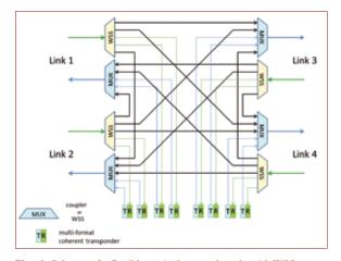
**Fig. 4:** Scheme of a flexible optical network node with WSS-based ROADM architecture.
