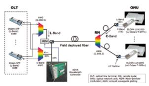
Fig. 5: Experimental set-up of tunable DWDM-PON system with central wavelength control.
