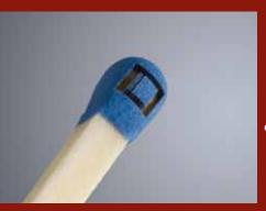
Fig 1: Engraved safety match demonstrating cold ablation by ultrashort laser pulses. Source: TRUMPF.
