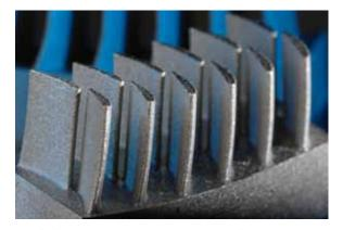
**Fig. 3:** Complex micro component, made with Selective Laser Melting. Source: Fraunhofer ILT, Aachen.
