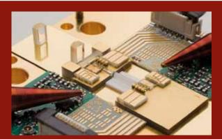
ps light source with DBR laser und GaN amplifier, suited as seed laser for materials processing. Source: ©FBH/schurian.com
