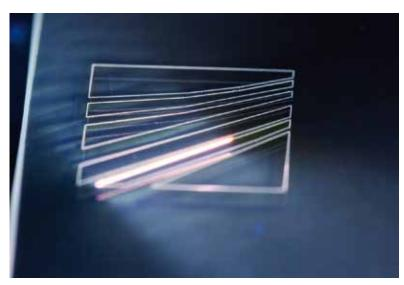
Cutting of thin glass with an ultrafast laser. Source: Fraunhofer ILT. Aachen.
