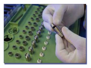
Fig.4: Assembly of Micro Annular Gear Pumps Source: HNP Mikrosysteme GmbH
