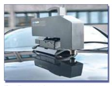
**Fig.1:** The optical 3D surface inspection is ideal both for the lab as well as demanding industrial use, e.g. for checking paint appearance in the automotive industry. (Photo: NanoFocus)
