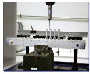
**Figure 3:** : Sensoric workpiece carrier on a coordinate measurement machine [Kugler, 2015].
