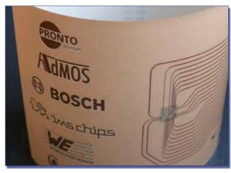
Fig. 3: ULTIMUM demonstrator, Chip embedded in liquid crystal polymer
