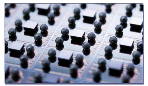
Fig.2: Chip-to-Wafer Stock for 3D Integration. Source: © Fraunhofer IZM
