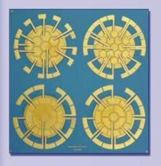
Figure 1: Different layouts of PZT thick film actuators on LTCC substrate used as adaptive mirrors for laser beam shaping (FhG IKTS/IOF)
