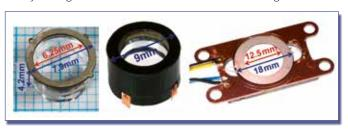
Fig. 3: Images of elastomer and fluid lens.
