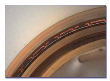
Fig. 1: Ultra-thin chips embedded in liquid crystal polymer
